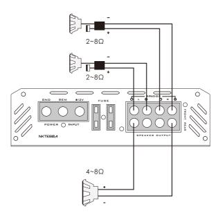
Caution:3CH mode conect the subwoofer to the channel switch with "LPF"
