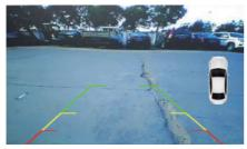
After the vehicle is put into R gear, the system interface displays a reverse camera screen.
